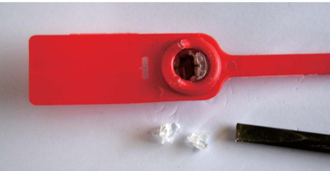
The cap is made with fragile material it is easy to be broken once prizing.
